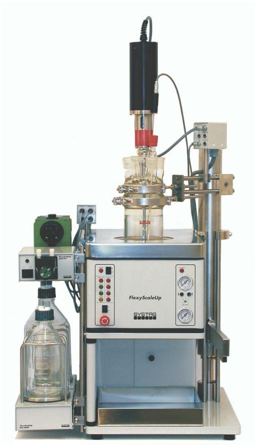
1.3 l reactor (with jacket adapter) and 2 dosages with membrane and peristaltic pumps, propeller stirrer and gas tight magnetic coupling, speed 36 - 1800 rpm, torque up to 75 Ncm.
