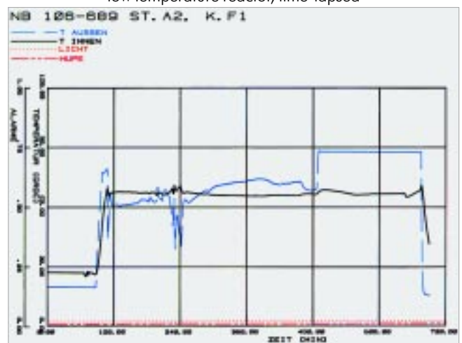
Figure 4: Manually controlled reaction in a low temperature reactor, time-lapsed
